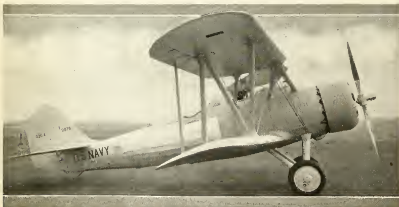
Vought "Corsair" powered with the new "Twin Wasp Junior" engine
